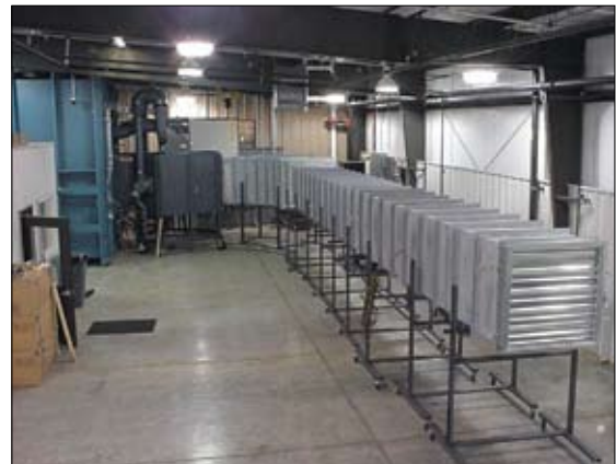
Greenheck's UL Certified on-site testing lab utilizes heated air capabilities to simulate fire emergency conditions required by new UL Standards for Fire Life Safety Dampers.
