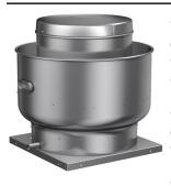
The CUBE is an aluminum exhaust fan specifically designed for roof or sidewall mounted applications where contaminated or grease laden exhaust air can be discharged directly upward, away from the roof or wall surface. The fans feature a one piece windband continuously welded to curb cap and double studded isolators for true vibration isolation.
